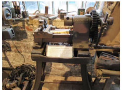
Among the larger items was a hand operated pedestal drill and a threading machine which would have been used for cutting threads for bolt (for screws). The lath and plaster ceiling had been left intact, due to the building being listed.
